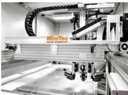
The laser welding unit is a fully-automatic machine with modern CNC control.
