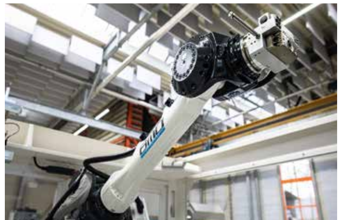
A Yaskawa 6-axis robot assists by loading the CNC machine.
