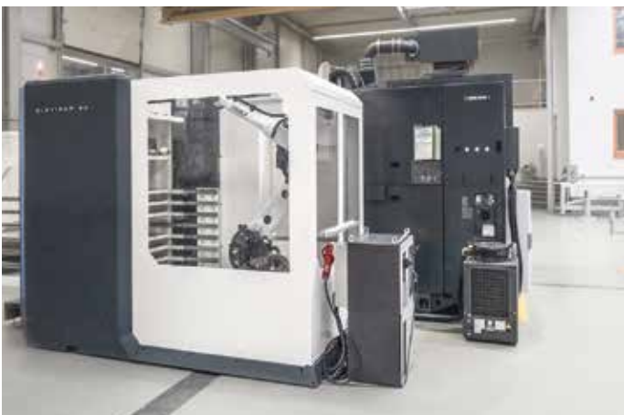
Recently put into operation: A robot cell for loading an existing CNC machine with workpieces automatically
