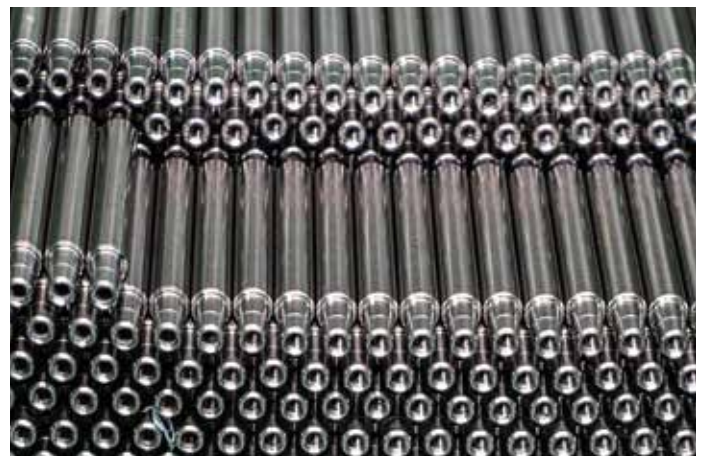
Smaller, edge-zone hardened precision steel shafts can now be produced in larger quantities on attractive terms.
