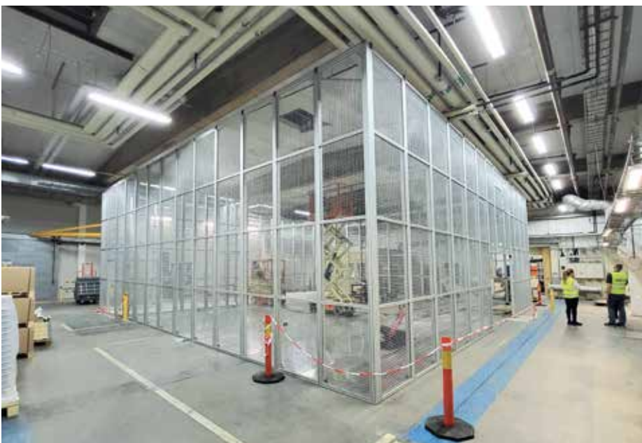
From the MiniTec modular system: XXL protective enclosure for a system for checking submarine cables for possible damage.
