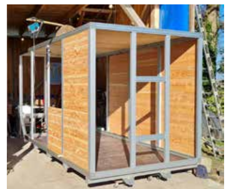
Campers with flexible fitout possibilities and a stable aluminium frame.
