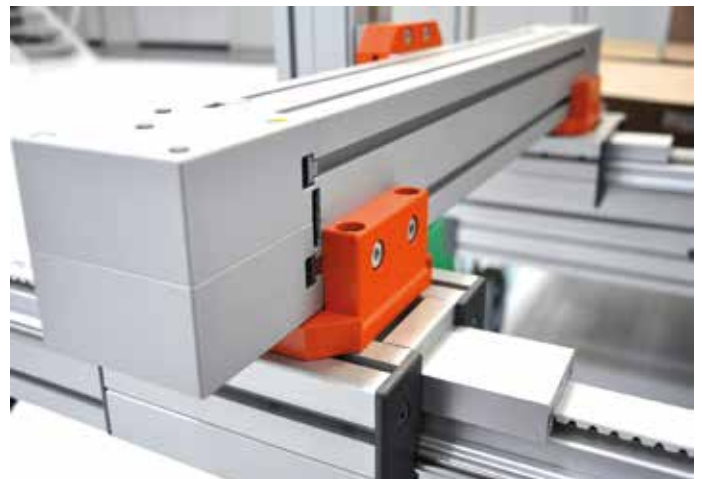
Linear axes can be combined with adapter plates (orange in the image).
